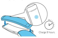
Charge your handset by docking it in either direction. The LED at the back of the handset flashes once.
